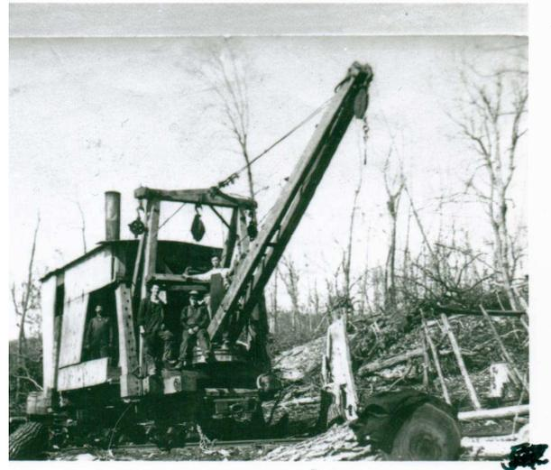
A Surry-Parker log loader, probably owned by the lumber company, at work in the mountains. These machines were popular in areas where lighter weight trees did not require a heavy-weight steel loader (notice its wood framework). You can see the devastation that clear-cutting can wreak in the background.
