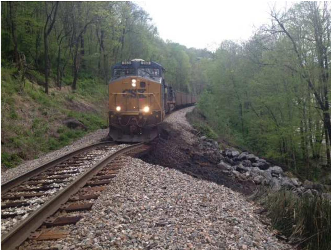
Mike Tilley sends along this May 7<sup>th</sup> photo by T. Hill of a bad slide on the Blue Ridge Subdivision of CSX (ex-CLINCHFIELD) at Mile Post 166, proof of the dangers of railroading even in these modern times. You can see the front wheels of the lead engine resting on rails, hovering over a 10 foot slide. Fortunately, the rail supported the engine and did not break. Disaster was averted by the crew getting in the back
