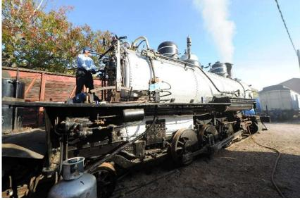
The contractor rebuilding Chesapeake & Ohio 2-6-6-2 No. 1309 recently issued a detailed status report on its work, but did not say when the locomotive would be ready for service. The restoration is being undertaken at the Western Maryland Scenic Railroad where the locomotive is based. **Diversified Rail Services said** of 36 the top row superheaters have been installed, the cab floor, stoker elevator tube, and grate
