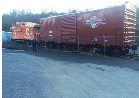
**C&O CABOOSE 903103:** The caboose project is about finished. The exterior has been repainted and decals Handle with Care are back on the caboose. Work is on going on the interior with painting presently going on now.
