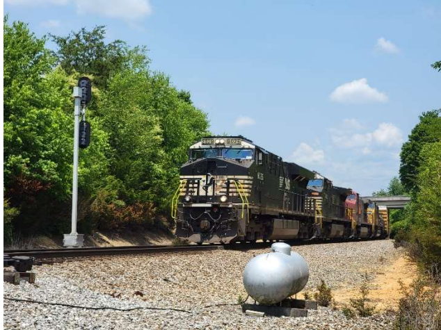
[Above] Piney Flats – NS 127 pulling into C.P. Curtis moving past the propane tank for wintertime thawing of the switch. It was headed toward the siding to wait on an eastbound.
