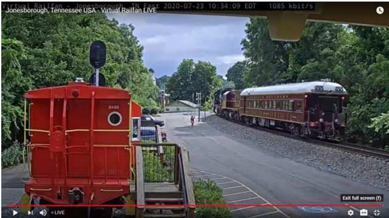
There's quite a variety of rail traffic to be seen when viewing the Historic Chuckey Depot live webcam. Here we see Norfolk Southern's Geometry Train, with unit NS 38, commonly known as "The Brick", and research car NS 36 in tow. Colorful beams of light from the bottom of the cars take a digital profile of the track which is then used for future maintenance and upgrades.
